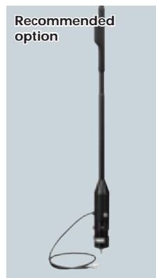
AT230 AUTOMATIC TUNING ANTENNA (Moonraker Australia Pty. Limited) 2.6m (8.5ft) length mobile mount whip antenna covers 2–30MHz with automatic tuning function. Continuous CW transmission at high power not guaranteed with AT230.
